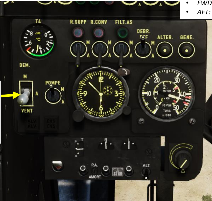
Starter/Ventilation (Démarreur) Switch M = Marche = ON (UP) A = Arrêt = OFF (MIDDLE) VENT = Ventilation, Dry Crank (DOWN)
